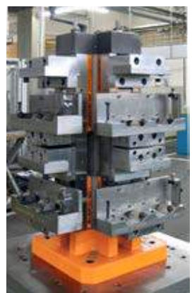
Special design of Monoblock DUO 125 4 x 90° for machining complex cast parts
