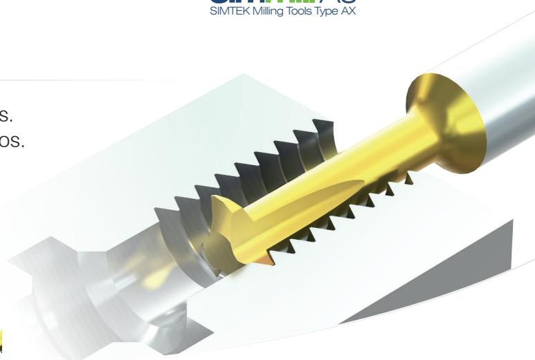
Solid micro grain carbide milling cutter for groove milling applications in bores as of min. Ø 0.055" (1,4mm). Available with three and partly with four cutting edges. High groove depths as well as extended thread depths at low cutting pressure are possible with this system. Wide range of standard applications.
