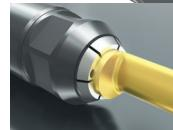
Very precise and strong tool system of solid carbide cutting insert and steel toolholders. High repeat accuracy from insert to insert and usable lengths up to 9xD! For best performances in bores between Ø 0.012" (0,3mm) up to Ø 0.315" (8,0mm). More than 3,000 standard items provide the right answer for almost every internal turning application.
